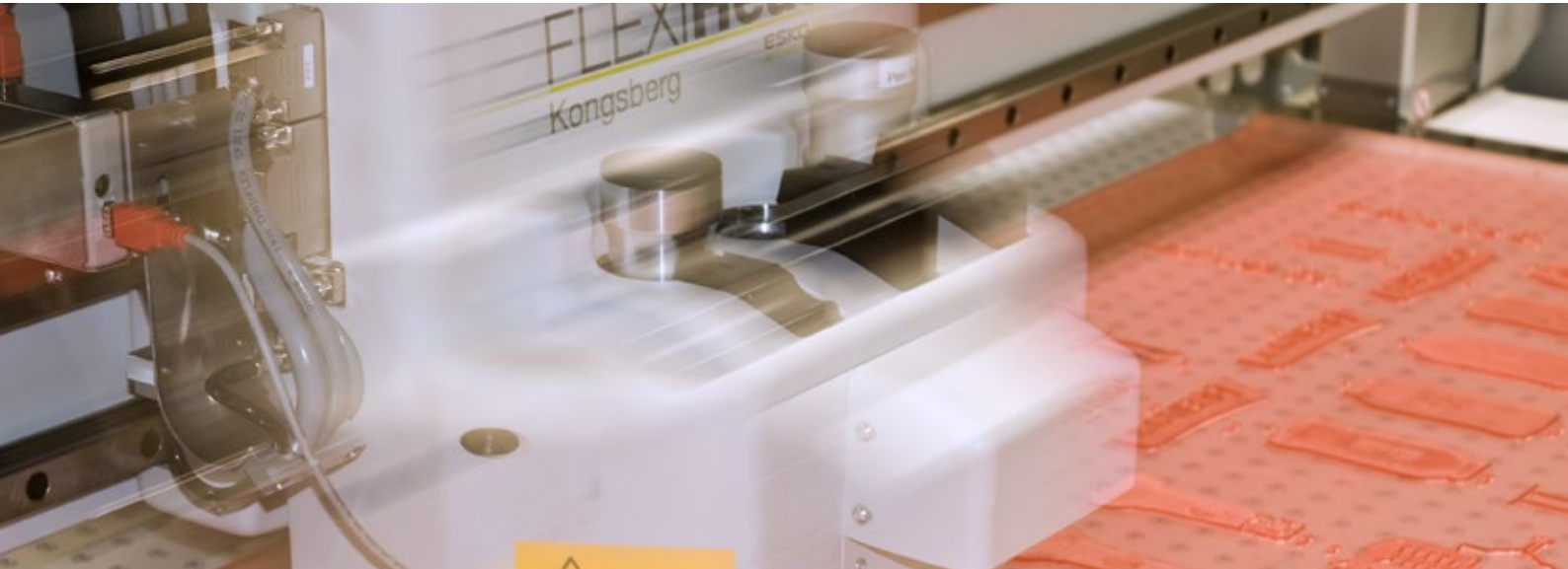
Kongsberg digital cutting tables cut the flexo plates quickly and accurately.
