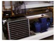
Integrated heater-chiller for solvent temperature control, solid content measurement and solvent replenishment.
