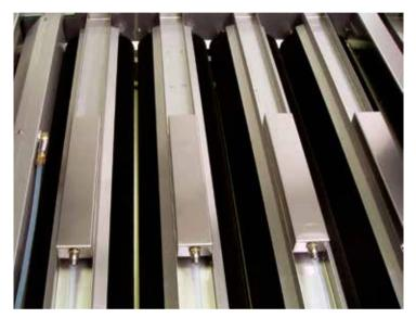
The unique brush movement reduces the processing time and eliminates any kind of movement of the plate when in contact with the brushes.
